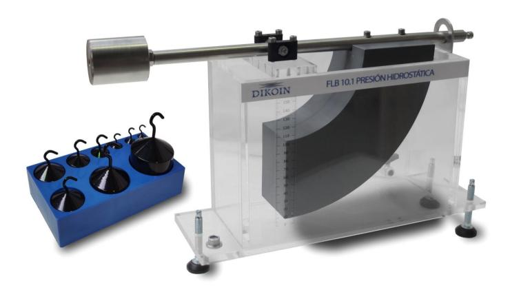
This equipment is designed for the study of the pressure exerted by a fluid on a surface submerged in it.
